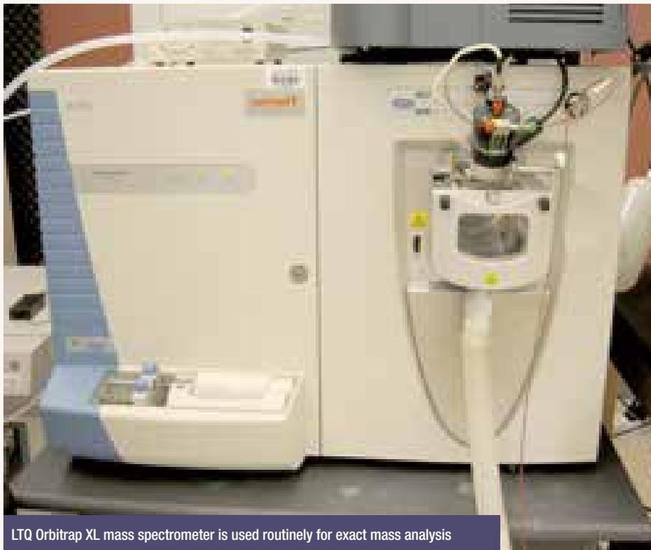
LTQ Orbitrap XL mass spectrometer is used routinely for exact mass analysis
