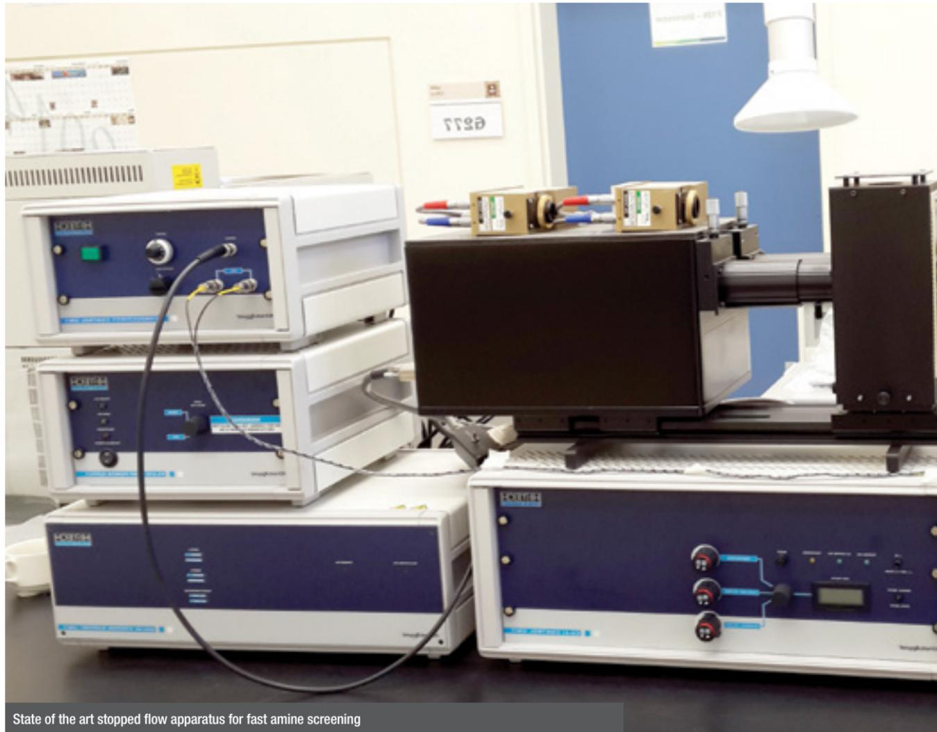
State of the art stopped flow apparatus for fast amine screening
