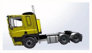
Figure 3. Installation of the smokeless exhaust tube onboard a truck.
