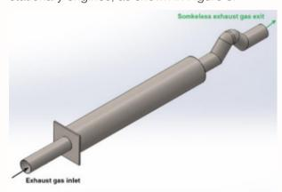
Figure 1. The smokeless exhaust tube.
