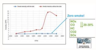
Figure 2. Measurements of the smoke intensity of a diesel engine with and without using the tube.
