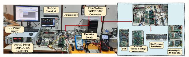
Figure 2. The developed converter for low-speed electric vehicles.
